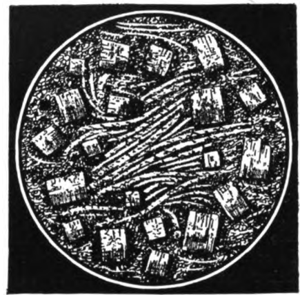
A magnified view of a coarse-grained anti-friction metal
